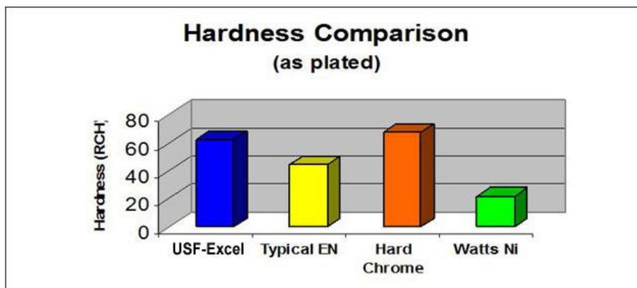
Often times heat-treating is not possible. Some substrates can't be subjected to these high temperatures due to impact on critical tolerances and/or effect on surface hardness of the components. In some cases heat-treating can be impossible due to size constraints and is often time consuming. In addition to this, heat treating increases the cost of the process. **USF-Excel** is an alternative.
