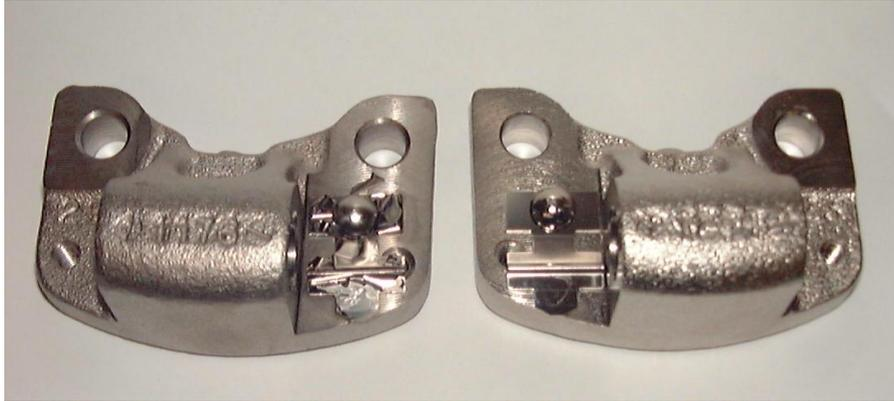
In addition to the aforementioned advantages, compressive stress deposits like the **USF-Excel** will not reduce the fatigue strength of the plated component, thus ensuring its possible use in aerospace applications.
